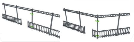
2) Keep bending by 45degrees along each pole as seen below:
