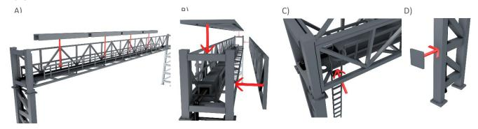
9) Lastly glue the ladder and as show above in image C. Add the number plate to one of the legs as seen in image D. You can also add the Overhead line equipment to any track that requires it. Once complete wire this up to your chosen controller.
