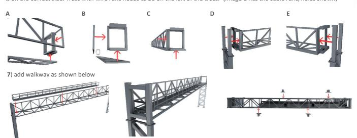
8) Glue the ASP hoods into locations as shown in the image above on the right. Feed wires along one side of the walkway and into the wire runs down the leg. Add cable cover as shown below in A, then glue final 2 parts of the gantry into place as shown in B.
