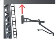
10) Lastly Glue the ladders on as shown. (You will need to bend ladder as shown below, heat can be used or it can be done
