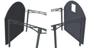
2) Glue roof trussing to the tops of the truss legs as shown below:
