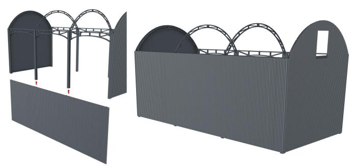
The imagery below shows how the back panel slots into the truss legs near the base. The panel still needs to be glued.
