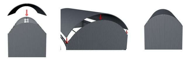
6) In this last step you need to add the guttering as shown below:
