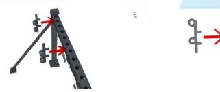
Finally glue the APT wire holder to the side of the structure. Again, no need to mount if no using an auto transformer model in an overlap section. However, it can make thigs look more details if used. (Image E)
