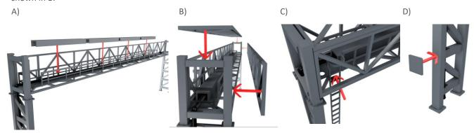
9) Lastly glue the ladder and as show above in image C. Add the number plate to one of the legs as seen in image D. You can also add the Overhead line equipment to any track that requires it. Once complete wire this up to your chosen controller.
