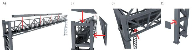
6) Lastly glue the ladder and as show above in image C. Add the number plate to one of the legs as seen in image D. You can also add Overhead line equipment to any track that requires it. Once complete wire this up to your chosen controller.
