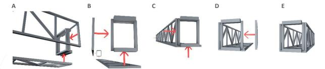
**4**). Attach gantry to legs as shown below: Note how the gantry mounting slots fit between those top poles.
